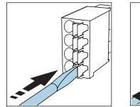
Press the screwdriver against the clip (opens the terminal).
