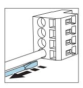
• Remove the screwdriver (closes the terminal).
