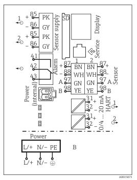
Overall wiring diagram BASE-E and
