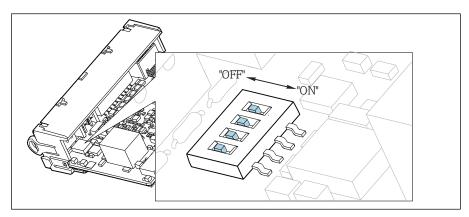
68 DIP switch for internal termination
