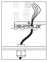
🗷 30 🛛 Tighten screw (2 Nm)
