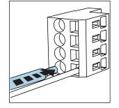
• Insert the cable until the limit stop.
