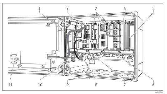
☑ 2 Example of a four-channel device with an open display cover (without wiring)
