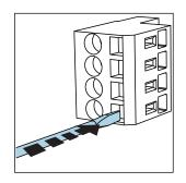
• Press the screwdriver against the clip (opens the terminal).
