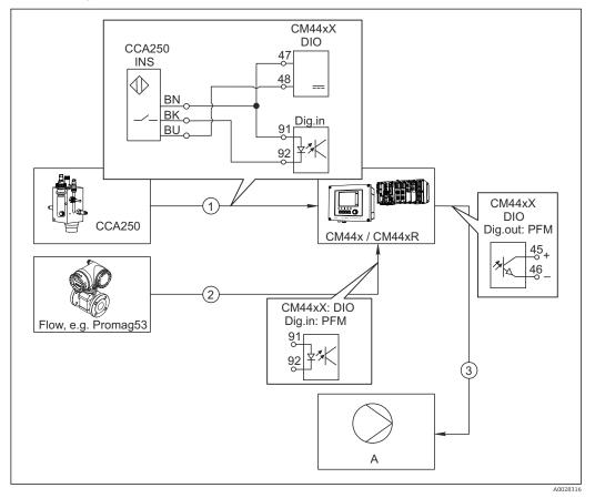
E 79 Example of chlorine control with feedforward control
