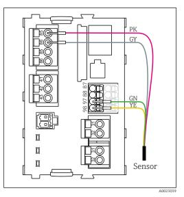
🖻 38 sensors with additional supply voltage
