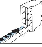
Insert the cable until the limit stop.
