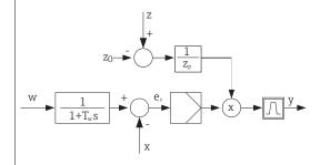
Strictly speaking, feedforward control involves an open-loop control system, since its effect is not measured directly. That means that the feed flow is directed exclusively forward. Hence the designation "feedforward control".
