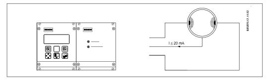
DC-cleaning is used to eliminate electrically conductive deposits in the measuring pipe influencing the measuring accuracy.
