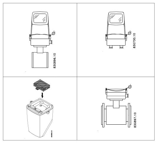
MAG 6000 CT is installed like a standard MAG 6000 except for the final sealing. Calibration sealing has been carried out at calibration.
