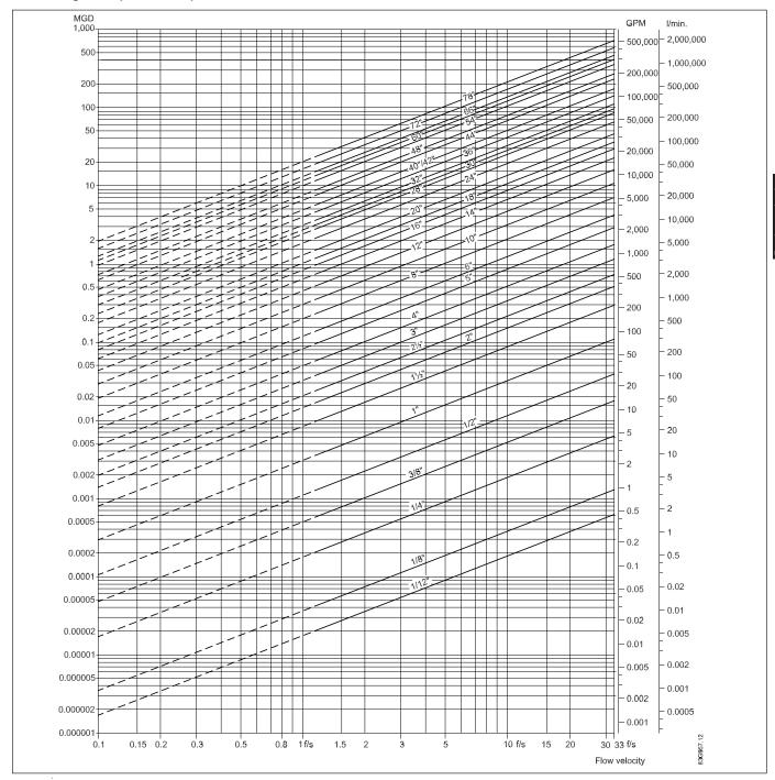
The table shows the relationship between flow velocity V, flow quantity Q and sensor dimension size.
