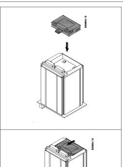
Locate the add-on module in the bottom of the MAG 6000 transmitter.
