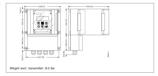
Wall mounting transmitter with cleaning unit or intrincically safe barrier
