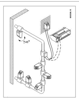
Reading and operating the flowmeter is possible under almost any installation conditions because the display can be oriented in relation to the sensor.
