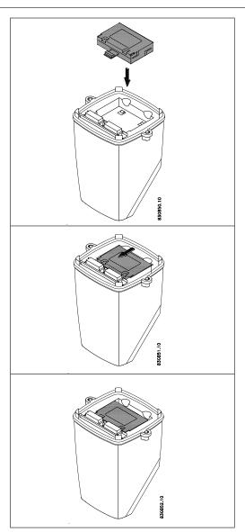
Locate the add-on module in the bottom of the MAG 6000 transmitter.
