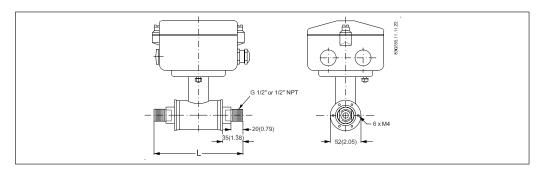
The MAG 1100  $^{1}/_{12}$ " and  $^{3}/_{8}$ " are prepared for assembly with the  $^{1}/_{2}$ " pipe connection.
