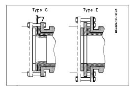
With abrasive liquids, flowmeter inlet protection may be necessary. Here type C and E grounding rings are used.
