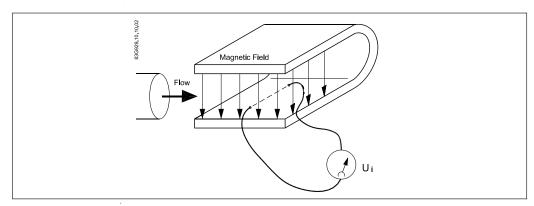
$U_i$  = When an electrical conductor of length L is moved at velocity v, perpendicular to the lines of flux through a magnetic field of strength B, the voltage  $U_i$  is induced at the ends of the conductor
