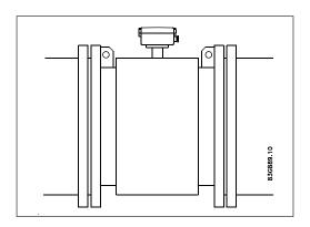
Potential equalization is carried out with the built-in grounding electrodes. No further action need to be taken.
