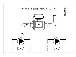
To achieve accurate flow measurement it is essential to have straight lengths of inlet and outlet pipes and a certain distance between pumps and valves.
