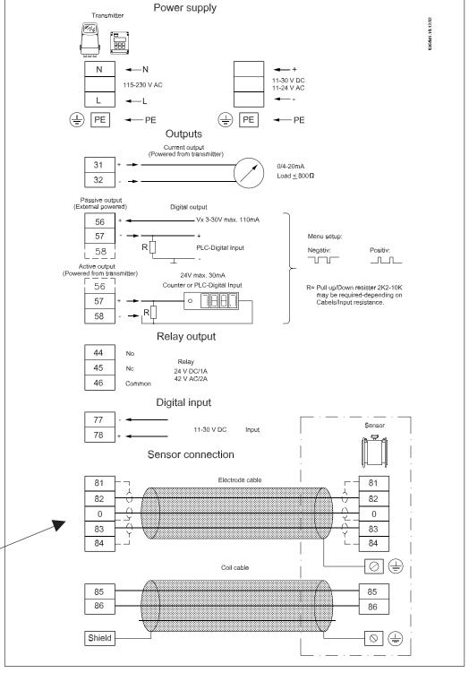
Special cable with individual wire shields (shown with dashed lines) are only required when using empty pipe function with low conductivity process (see "Specifications, chapter 2)
