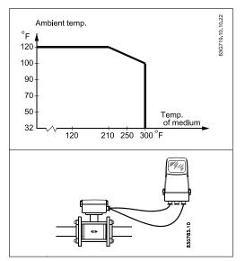
The sensor and transmitter can be installed either integral mount or remote.
