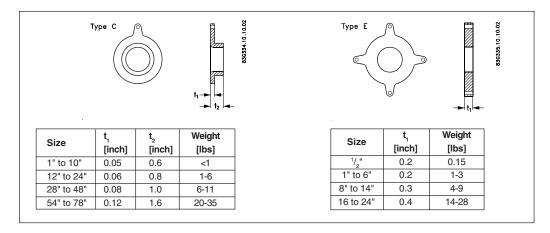
Type C flanges for liners of neoprene, EPDM, Linatex® and ebonite. Type E flanges for liners of PTFE.
