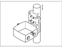
Mount the wall mounting on a vertical or horizontal pipe using an ordinary hose clamp or a duct strap.
