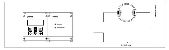
AC-cleaning is used to remove fatty deposits on the electrodes. Fatty deposits are seen from Slaughter houses and in rare instances from wastewater applications and water applications with oil residuals. During the cleaning process, the surface of the electrodes get warmer, which tends to soften grease particles and the gas bubbles generated mechanically lift deposits away from the surface of the electrodes.
