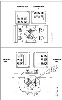
The transmitter can be mounted in either direction as the arrow indicates without turning the terminal box.
