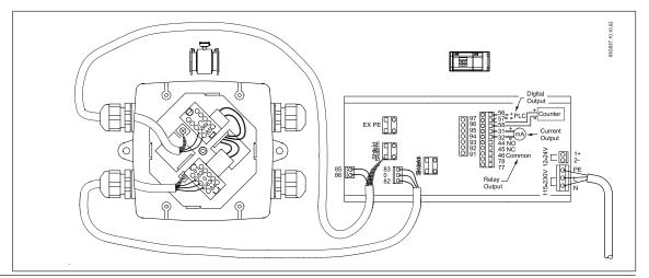
7.2.6 Wall mount with safety barrier NEMA 6 EEx (ia/ib) up to 12"
