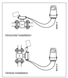
If the sensor is going to be buried or permanently submerged, the terminal box must be encapsulated with silicon dielectric gel. The optional kit has two components.
