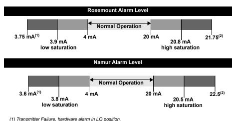
(1) Transmitter Failure, hardware alarm in LO position. (2) Transmitter Failure, hardware alarm in HI position.
