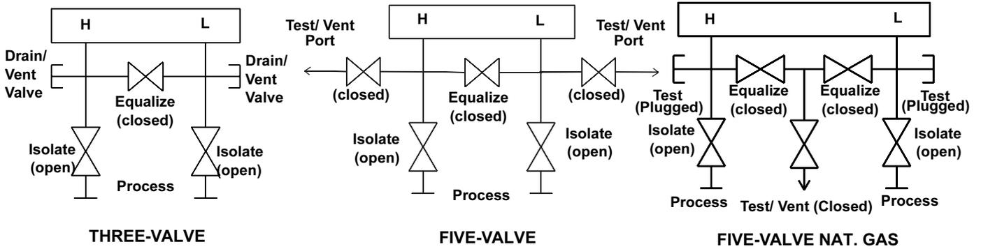
To check zero the 3095FB, close the block valve to the low pressure (downstream side) of the transmitter first.
