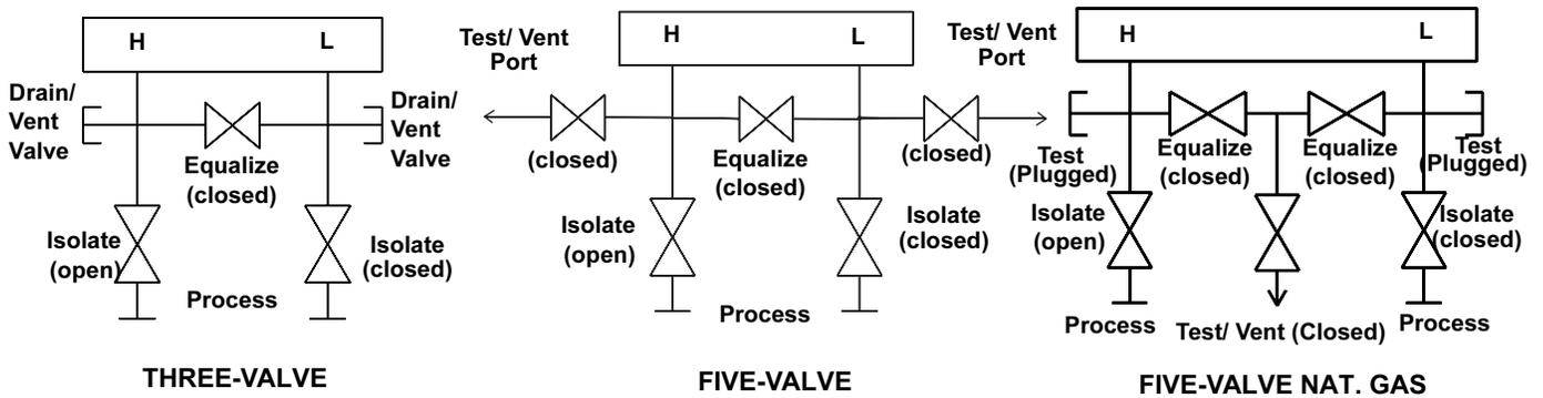
Next, open the center (equalize) valve(s) to equalize the pressure on both sides of the transmitter.
