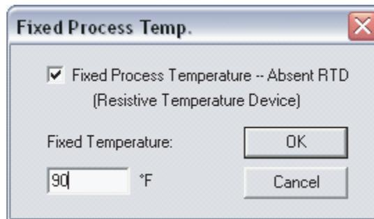
The 3095FB can be configured so that a user-selected temperature will be used as the process temperature measurement if an RTD failure occurs.
