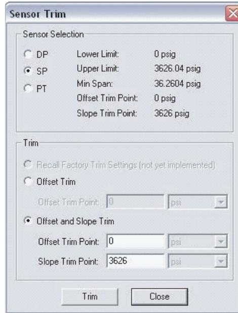
2. SP Offset (zero) and Slope (span) Trim
