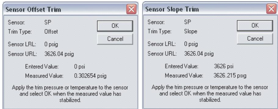
3. DP Offset (zero) and Slope (span) Trim
