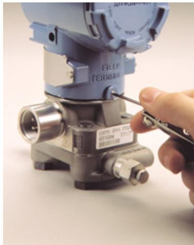
3. Unscrew the housing from the module, making sure the shroud and sensor cable do not catch on the housing. Damage can occur to the cable if the internal shroud and sensor cable rotate with the housing. Carefully pull the shroud and sensor ribbon cable assembly through the housing opening.
