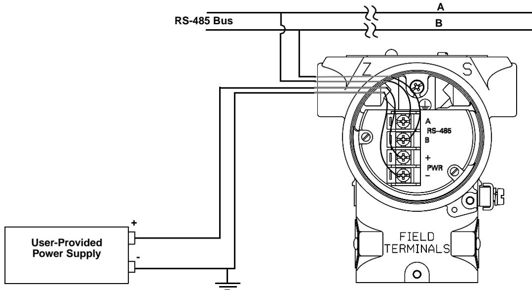
Inductive-based transient protectors, including the Rosemount 470, can adversely affect the output of the 3095FB transmitter. Do not use the Rosemount 470 for transient protection with the 3095FB. If your application requires transient protection, install the Transient Protection Terminal Block (Section 5: Troubleshooting).
