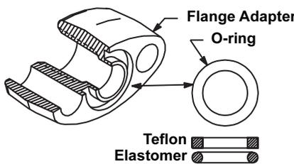
Refer to the Spare Parts list on page A-9 for the correct part numbers of the flange adapters and O-rings designed for Rosemount 3051 transmitters.
