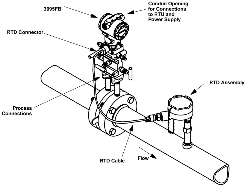
The 3095FB transmitter total weight varies depending on the components ordered (see Table 2-1). This weight must be securely supported.
