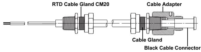
1. Fully engage the black cable connector to the 3095 RTD connector (figure 2-9).
