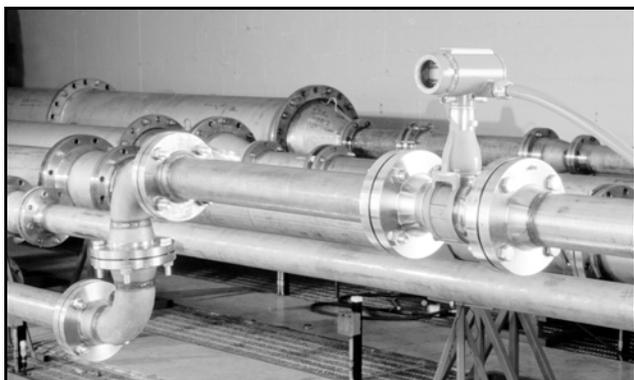
One of the perceived limitations of vortex meters is that they are highly sensitive to installation effects. Since it is true that the conditions in a plant environment may be quite different than the conditions under which the vortex meter is calibrated, some meters may be adversely affected by the installation conditions. The Rosemount® 8800 Vortex Flowmeter is designed to compensate for or limit the effects encountered in actual installations.
