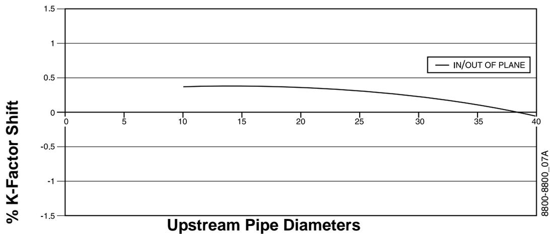
FIGURE 4. Double Elbow in Plane
