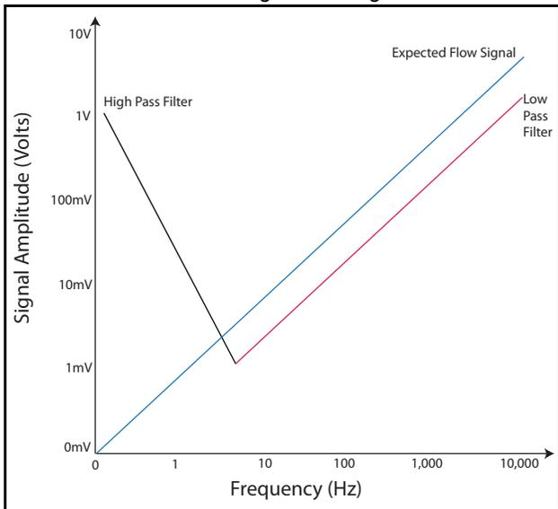
Figure 4 illustrates the placement of the Low Pass and High Pass Filters in relation to the expected flow signal. The flow signal must be inside the “V” created by the Low Pass and High Pass Filters to be measured as flow.
