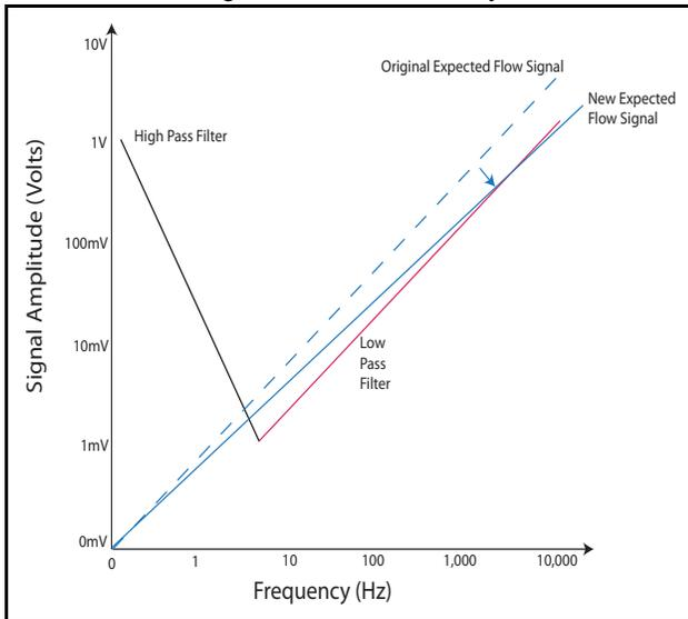
Figure 17 illustrates that if the filters are not adjusted to accommodate for the lower process density the 4:1 signal to trigger level ratio is not maintained and there is an increased possibility that flow measurement will become noisy or lost entirely.
