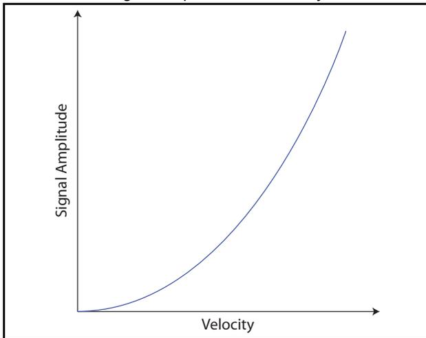
The vortices must be able to transfer enough force or energy to the sensor for it to measure their generated frequency. The term of  $\rho V^2$  in Equation (12) is actually a measure of energy in the flow stream as it relates to kinetic energy.
