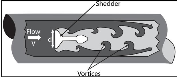
As a fluid passes by a blunt surface (Shedder), the fluid separates and forms areas of alternating differential pressure (Vortices) around the back side of the blunt surface. The frequency of the alternating vortices is linearly proportional to the velocity of the fluid.
