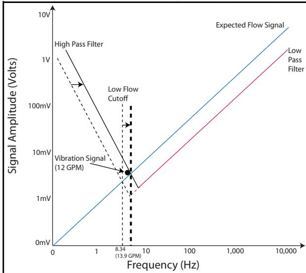
Figure 26 shows the filter settings with the low flow cutoff adjusted upward above the false flow indication. As stated in “Low Flow Cutoff” on page 17 the low flow cutoff can be adjusted in 18% steps. In this example, two steps of adjustment were required. The goal of adjusting the low flow cutoff is to eliminate the false flow indication caused by pipe vibration without cutting into the desired measurable range.
