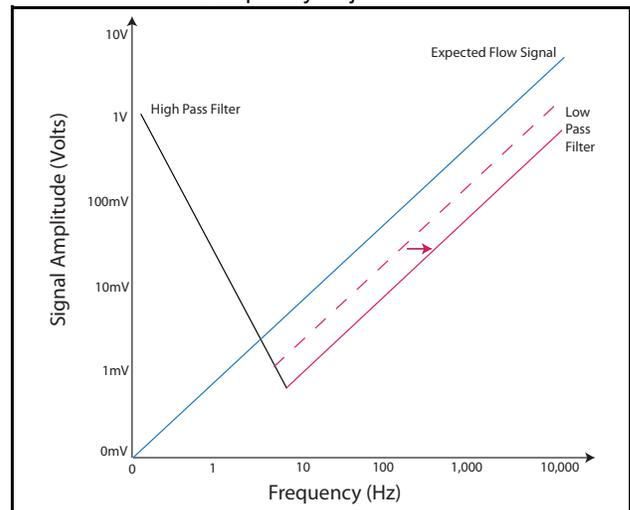
Figure 19 illustrates an increase in the Low Pass Corner Frequency. The increase shifts the Low Pass Filter to the right.
