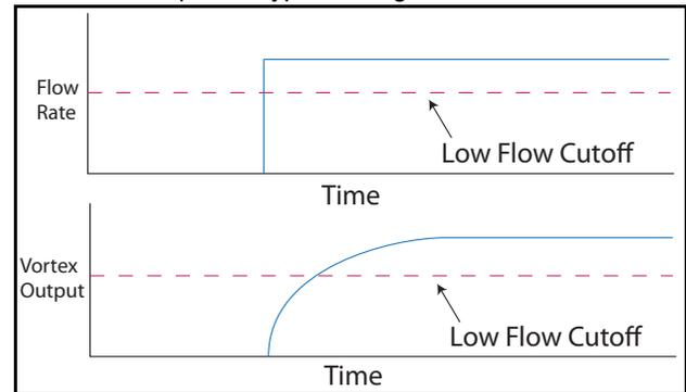
Figure 11 shows the flow rate starting at zero and then making a step change to a flow rate that is greater than the Low Flow Cutoff setting. With the LFC Response Type set to damped, the output will start at zero and ramp up to measured flow rate.
