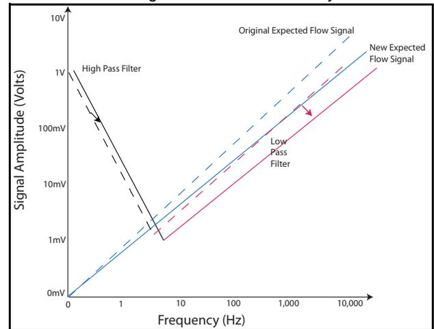
Figure 18 illustrates that the Auto Adjust Filter function has moved the filter “V” to retain at least the 4:1 signal amplitude to trigger level based on the new process density.
