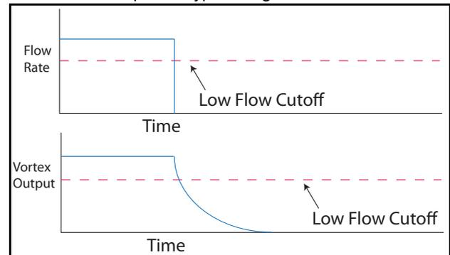
Figure 12 shows the flow rate starting at flow rate above the Low Flow Cutoff setting and then making a step change to zero flow. With the LFC Response Type set to damped, the output will ramp down to zero and there will be a period of time when the output is below the Low Flow Cutoff value.
