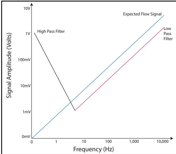
The actual process density was lower than originally expected. A lower process density would lead to lower signal amplitude as stated in the Vortex Signal Amplitude/Strength section.
