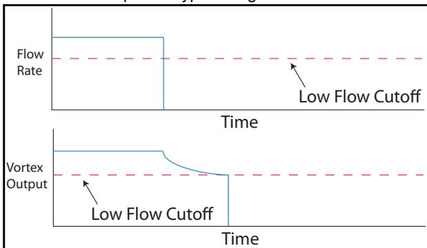
Figure 14 shows the flow rate starting at flow rate above the Low Flow Cutoff setting and then making a step change to zero flow. With the LFC Response Type set to stepped, the output will start to ramp down to zero but once it gets to the Low Flow Cutoff setting it will jump directly to a zero flow output.
