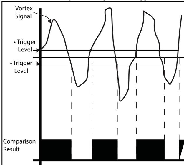
Figure 10 shows a noisy vortex signal superimposed on the threshold limit or trigger level.
